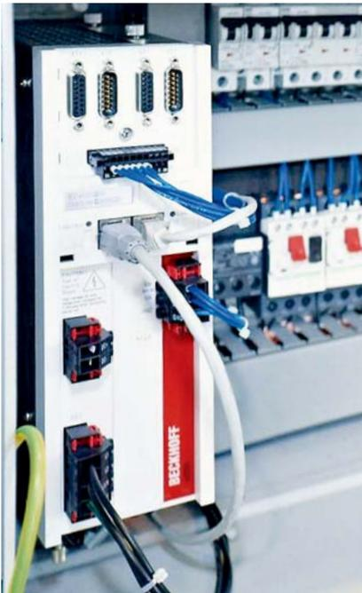
With the TwinSAFE terminals (left) and the EL7201 servomotor EtherCAT Terminal (right), extremely compact safety and drive technology can be integrated seamlessly into the control system.
