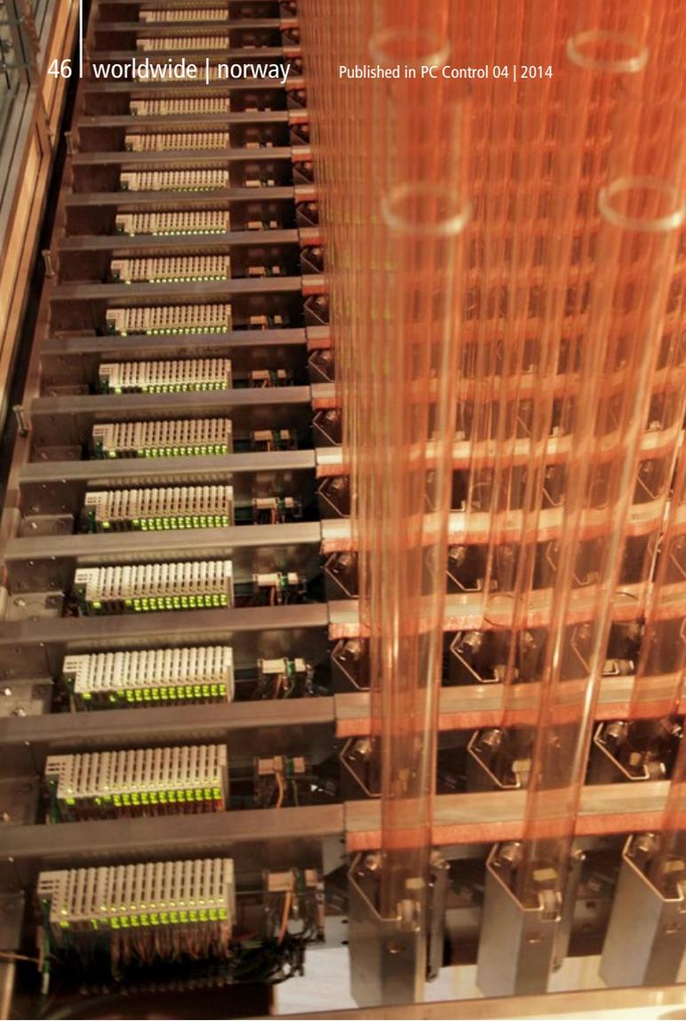
The compact electronics that control the 529 plexiglas tubes are installed at both ends of the support structure. The controls consist of an EK1100 EtherCAT Coupler, digital input terminals, servo terminals, and buffer capacitor terminals.
