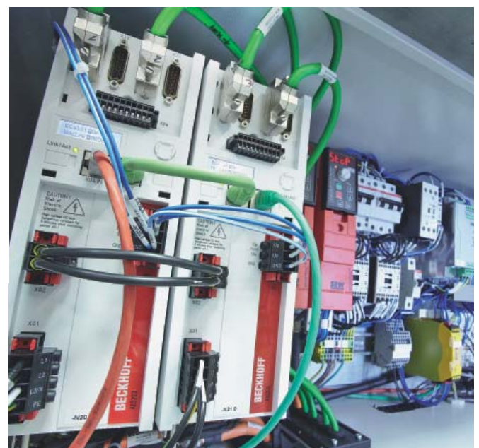
View inside the control cabinet, with EtherCAT AX5000 Servo Drives and EtherCAT Terminals for the dynamic, reliable control of the delta robot.
