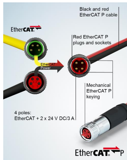
Figure 2: M8 P-coded connector and cable
