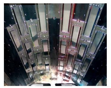
The Techma 4 printing machine has print heads arranged cubically to the print direction (left to right), as well as linearly to the print width (front to back). The control electronics on the Techma 4 are synchronized over EtherCAT and XFC.
