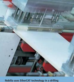
Nobilia uses EtherCAT technology in a drilling system for small and narrow components, and in a front drilling line as part of a drawer production line.
